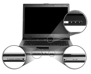
The power, battery and wireless communication status indicators are visible even when the LCD display is closed.
